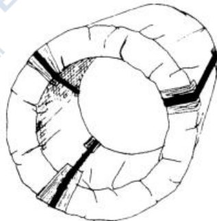
FIG. 87 Suitably Wrapped Individual Strip Coils or Groups of Coils
