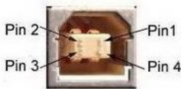
3.3.2 USB socket and pin definitions
