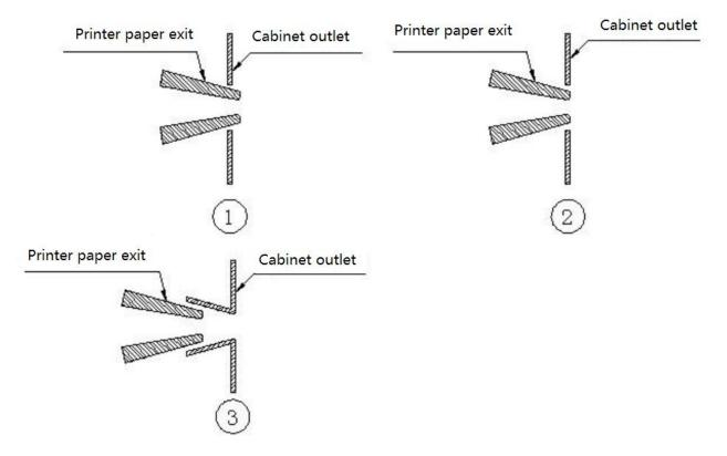
2. When the paper exit port and Cabinet outlet are connected in the above figure, in the structure of Figure 1 and Figure 2, there should be a gap between the paper exit of the printer and the paper exit of the device. See the figure below.
