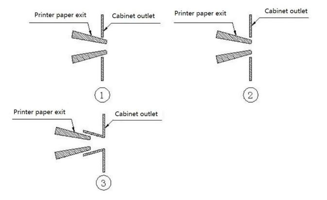
2. When the paper exit port and Cabinet outlet are connected in the above figure, in the structure of Figure 1 and Figure 2, there should be a gap between the paper exit of the printer and the paper exit of the device. See the figure below.
