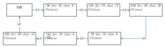
Dot matrix printer model can be alternatively choose through this setting:
