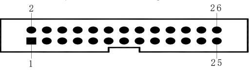
Figure 3-3 parallel interface socket pin number
