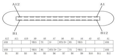
USB TO Type-C Socket and PIN Assignment
