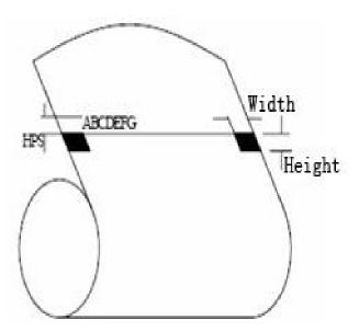
Printing Position: As the picture above, the black mark should be printed on the right or left edge of the side of words.
