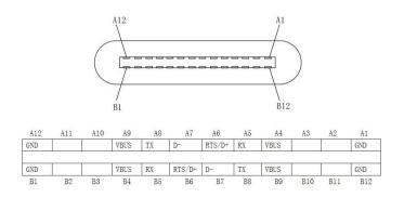
TXD: Printer send data to computer, when use X-ON/X-OFF handshaking protocol agreement, the printer will send control code X-ON/X-OFF to computer.
