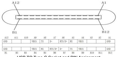
USB TO Type-C Socket and PIN Assignment
