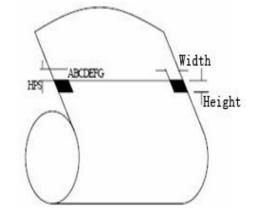
**Printing Position:** As the picture above, the black mark should be printed on the right edge of the printed side of paper.
