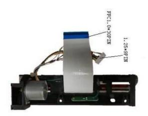
FFC1.0-30PIN ......Print mechanism wiring harness 1.25\*9PIN ......Motor and sensor wiring harness
