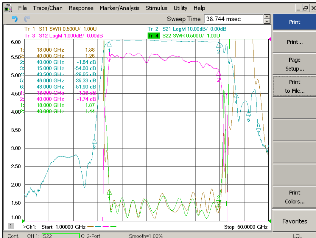
Figure 2 The sample test curve of the filter
