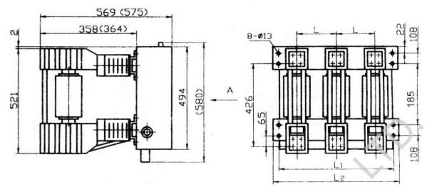
Note: (575) and (364) mean when short circuit breaking current is 40kA or above, the dimensions are 575mm, 364mm.
