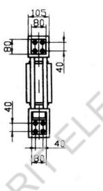
Upper and lower outlet terminal hole 4-M12
