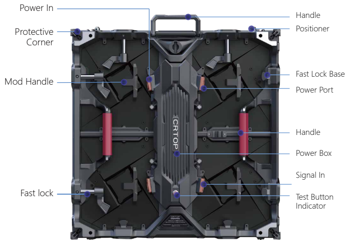
Cabinet size: 500*500*75mm Weight:7.8kg
