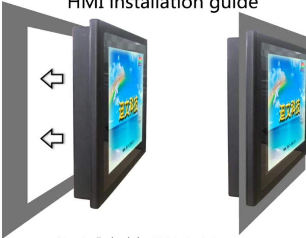
Step.1: Embed the HMI in the hole;
